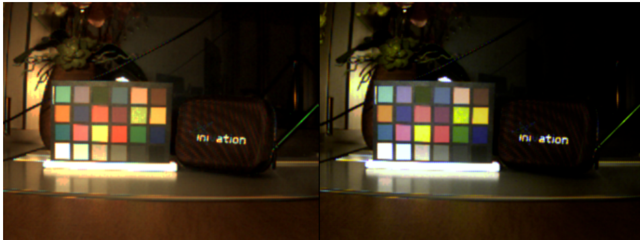
Original frame to the left and color corrected (post calibration) to the right.
