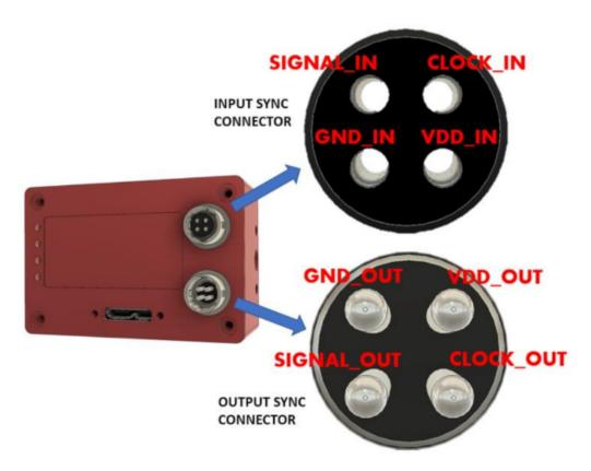
Input signals can be 3.3V or 5V, depending on the VDD\_IN supplied externally. **GND\_IN and VDD\_IN must always** be supplied.
