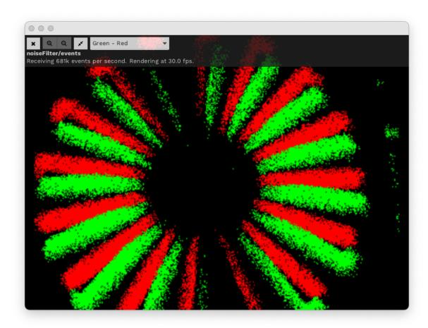
5. Adjust the focus ring until the pattern's centre is visible and sharp. Below is an example of the output with a focused
