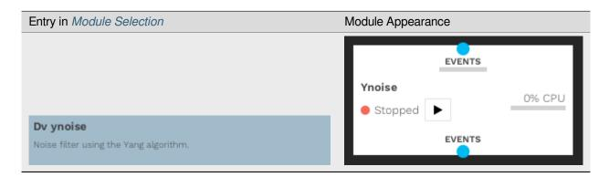
The Ynoise filter is based on the paper "Event Density Based Denoising Method for Dynamic Vision Sensor<sup>121</sup>", that describes a variant of the standard spatiotemporal filter.
