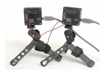
The signal on the IN pin has to be 3.3V. DO NOT connect this with devices providing a 5V signal, such as the DAVIS240! The OUT pin will always produce a 3.3V signal.
