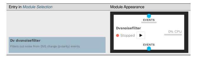
The Dysnoise filter is a standard spatiotemporal filter that stores a map of event timestamps. The filter also provides a hot-pixel filter with learning to filter "broken" (always-active) pixels in the sensor, as well as a refractory period filter, which limits the rate at which single pixels can consecutively generate events.
