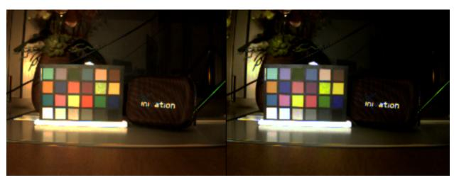
Original frame to the left and color corrected (post calibration) to the right.
