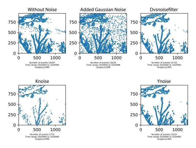
Note: data100k is an artificially generated event file without noise, data\_noise100k is that file with added Gaussian noise, and the other images are the output of the discussed filters.
