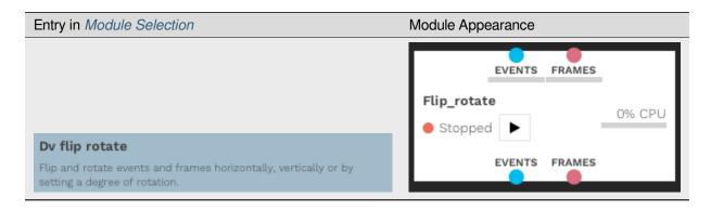
This module flips (vertically, horizontally) and/or rotates (-180° to 180°) events and/or frames.
