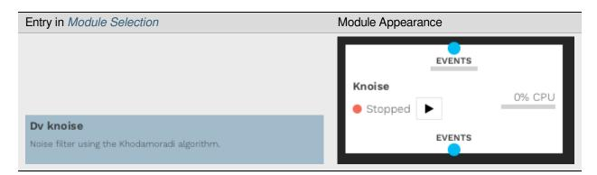
The Knoise filter is based on the paper "O(N)-Space Spatiotemporal Filter for Reducing Noise in Neuromorphic Vision Sensors<sup>119</sup>"; it is a spatiotemporal filter with memory optimizations. Memory usage and accesses are greatly reduced by only storing one timestamp per row and column.
