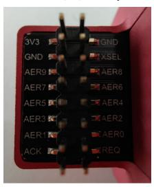
All data pins are 3.3V. A 3.3V reference and its Ground (GND) reference are provided on the connector. The 3.3V pin is only intended as a reference/output, do *not* power the device using this pin! The USB connector must be used always to provide power and configuration.
