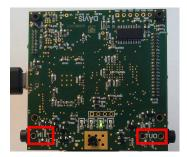
Any 3.5mm audio cable can be used to connect camers to each-other, and can be found at any AV store or suppliers such
