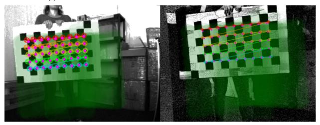
The option **Save Stereo Statistics** generates .csv files with the mean reprojected error of each acquired image from the two cameras.
