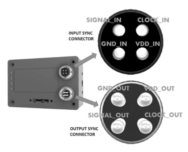
Synchronization connectors pinout is shown in the image above. Please note that all the pins in the SYNC IN ports are isolated from the SYNC OUT ports.
