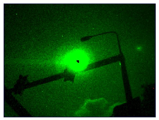
On the other hand, in dark conditions, noise is dominated by irregular ON and OFF events, which are more frequent from darker regions. The following image was created by accumulating all the ON and OFF events over several seconds whilst observing a rats nest of cables under a desk. In this case, the cables are black against a white wall, and produce more events. The additional events from a light to the bottom of the image are due to the light being driven by an oscillating current:
