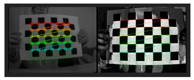
The area where a pattern has been found and added will turn slightly green. To get a good calibration result, one should cover the whole image in an even green shade. This can be turned off by unchecking the **Highlight Area** option.
