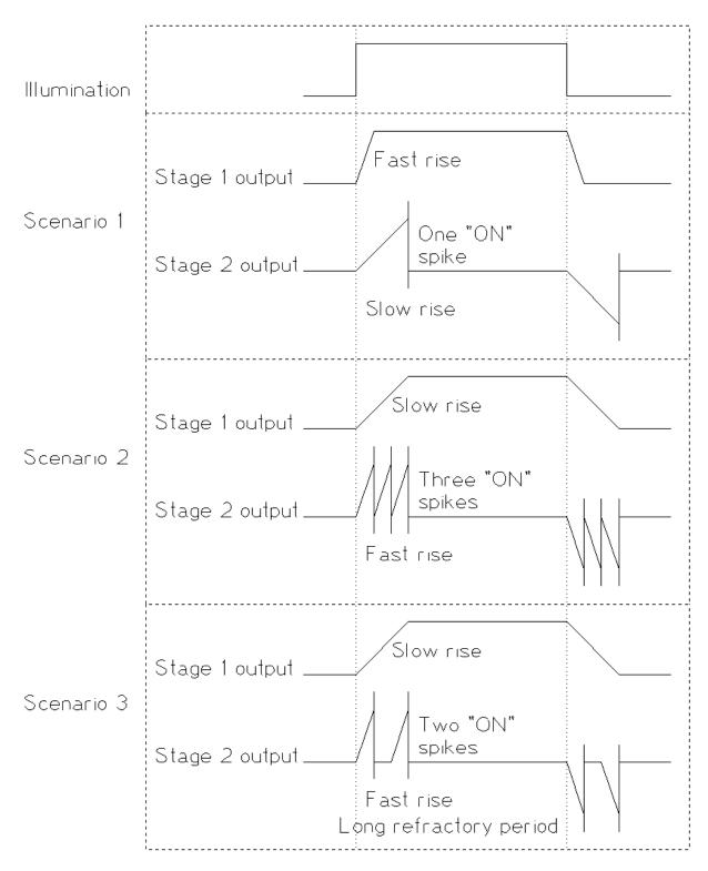
Let's assume that there is an instantaneous increase in light which is large enough to produce three threshold changes, given the choice of the biases which control the thresholds. There then follows a step back down. This is shown in "Illumination".
