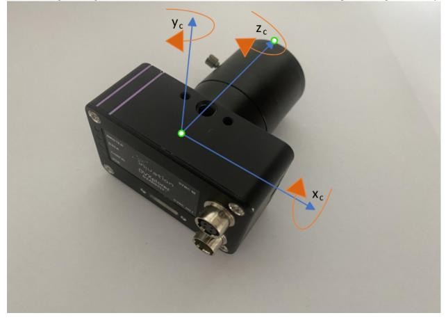
The image sensor uses the standard format: by looking at the camera from the back, X-axis points to the right, Y-axis up and Z-axis points towards the lens. In addition, the IMU axis are aligned with the camera one. The rotation for the gyroscope is counter-clockwise along the increasing axis, for all three axes. Note that, this does not follow the right-hand rule.
