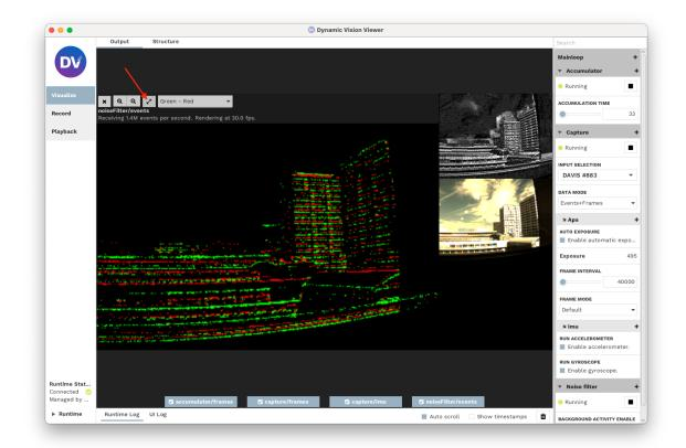
4. Start to rotate the focus ring on the lens. If you have a paper print out of the Siemens star, keep generating events by slightly jiggling either the camera or the pattern. At first, if the camera is out of focus, you might see something like the image below.
