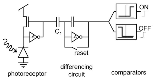
This shows that there are 3 parts of the DVS pixel:
