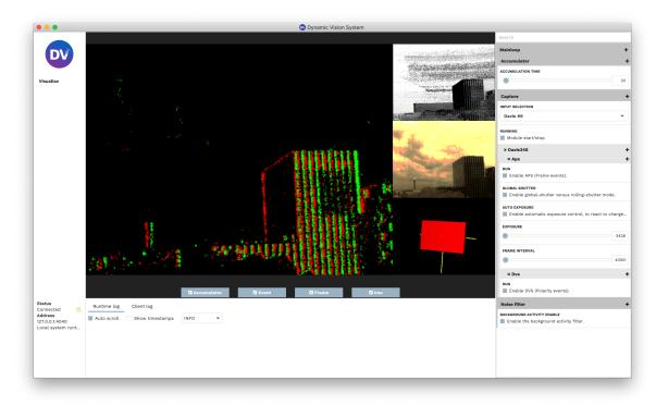
• The *runtime*, the backend of the GUI that takes care of all the processing logic. It is controlled via the GUI. Both of these components are made to work with *DV Modules*. Along with this software, we provide a library, *dv-sdk*, that allows users to extend the provided functionalities of the software or integrate their algorithms into it.
