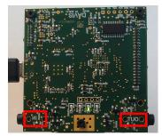
Any 3.5mm audio cable can be used to connect camers to each-other, and can be found at any AV store or suppliers such as digikey<sup>66</sup>.
