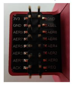
All data pins are 3.3V. A 3.3V reference and its Ground (GND) reference are provided on the connector. The 3.3V pin is only intended as a reference/output, do *not* power the device using this pin! The USB connector must be used always to provide power and configuration.
