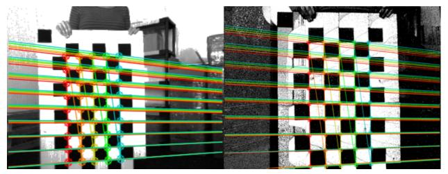
Another option for the stereo calibration is the possibility to draw the reprojected points from one camera to the other. You can select the **Draw reprojected points** option. This setting uses the Homography matrix (H) calculated during the calibration to map points from one camera to the other.
