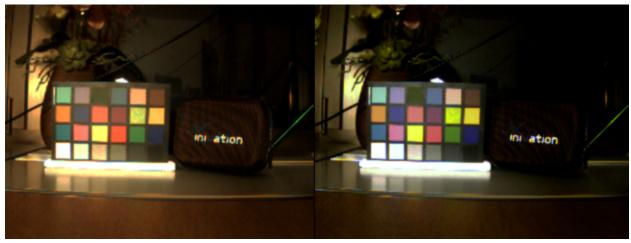
Original frame to the left and color corrected (post calibration) to the right.
