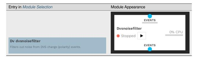
The Dvsnoise filter is a standard spatiotemporal filter that stores a map of event timestamps. The filter also provides a hot-pixel filter with learning to filter "broken" (always-active) pixels in the sensor, as well as a refractory period filter, which limits the rate at which single pixels can consecutively generate events.
