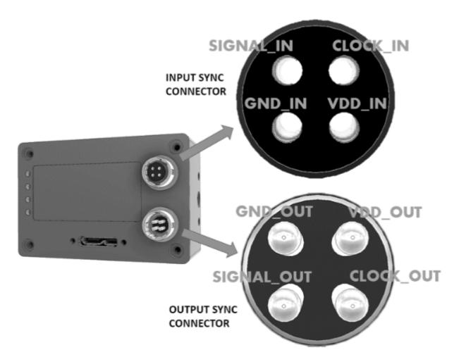
Synchronization connectors pinout is shown in the image above. Please note that all the pins in the SYNC IN ports are isolated from the SYNC OUT ports.
