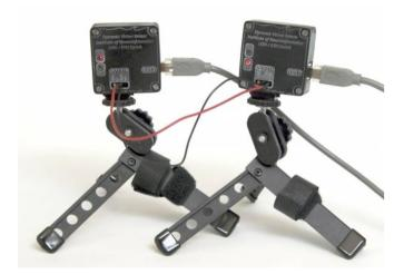
The signal on the IN pin has to be 3.3V. DO NOT connect this with devices providing a 5V signal, such as the DAVIS240! The OUT pin will always produce a 3.3V signal.
