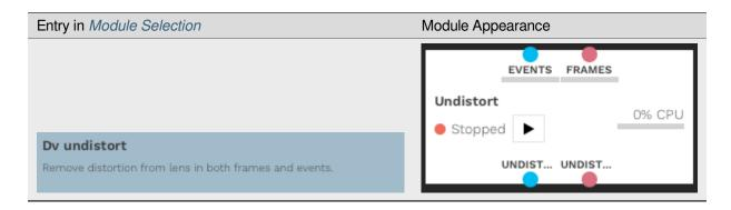
This module performs undistortion<sup>128</sup> on frames and/or events.
