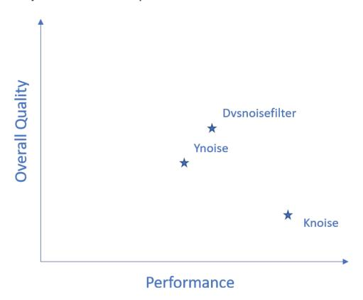
We recommend for standard usage (with static cameras or without significant scene changes) the Dvsnoise filter and the Ynoise filters. For dynamic camera situations or significant scene changes, we recommend the Knoise filter, as it is faster and will provide a better compromise for keeping good filter performance and real-time processing speeds.
