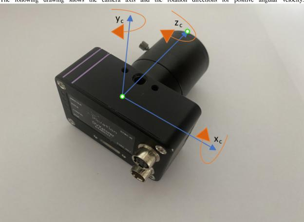
The image sensor uses the standard format: by looking at the camera from the back, X-axis points to the right, Y-axis up and Z-axis points towards the lens. In addition, the IMU axis are aligned with the camera one. The rotation for the gyroscope is counter-clockwise along the increasing axis, for all three axes. Note that, this does not follow the right-hand rule.
