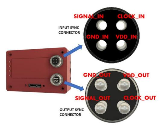
Input signals can be 3.3V or 5V, depending on the VDD\_IN supplied externally. **GND\_IN and VDD\_IN must always** be supplied.
