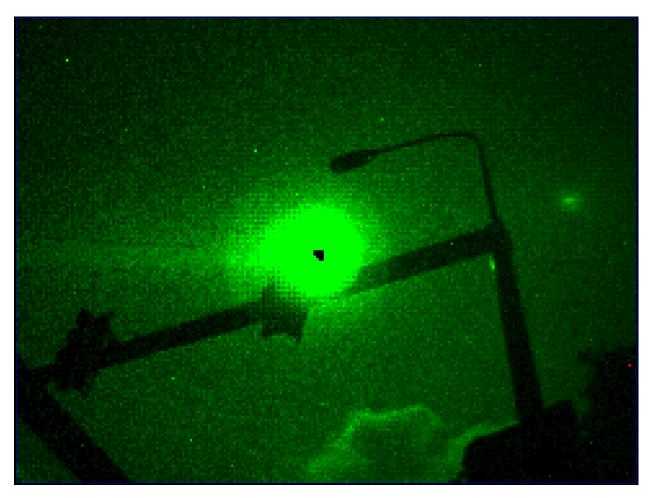
On the other hand, in dark conditions, noise is dominated by irregular ON and OFF events, which are more frequent from darker regions. The following image was created by accumulating all the ON and OFF events over several seconds whilst observing a rats nest of cables under a desk. In this case, the cables are black against a white wall, and produce more events. The additional events from a light to the bottom of the image are due to the light being driven by an oscillating current:
