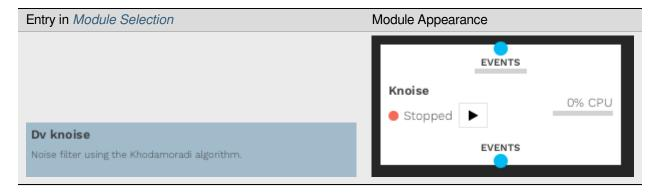
The Knoise filter is based on the paper "O(N)-Space Spatiotemporal Filter for Reducing Noise in Neuromorphic Vision Sensors<sup>119</sup>"; it is a spatiotemporal filter with memory optimizations. Memory usage and accesses are greatly reduced by only storing one timestamp per row and column.
