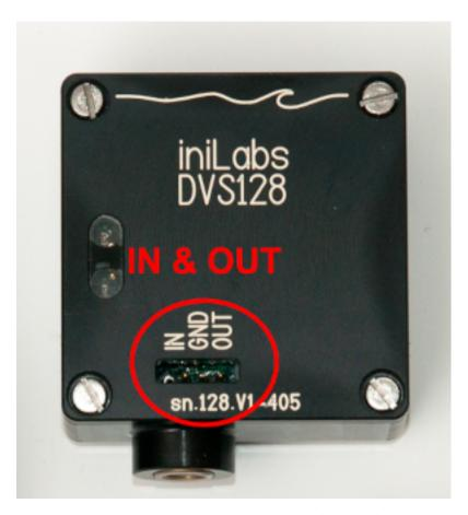
You can connect these using simple copper cables or jumper wire.
