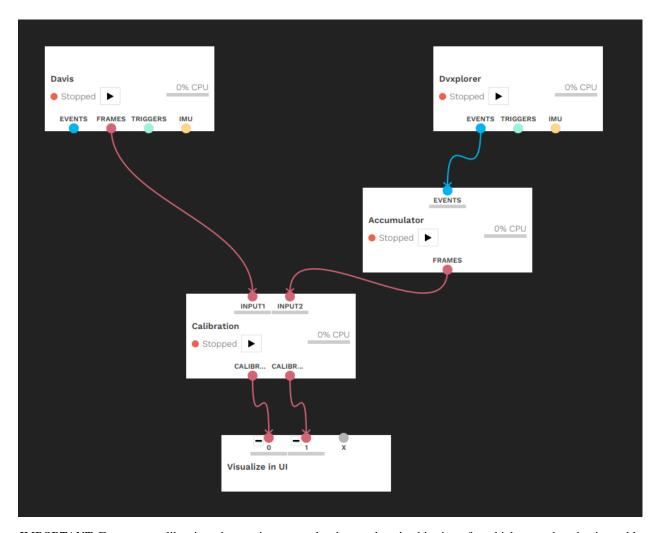
*IMPORTANT:* For stereo calibration, the two inputs need to be synchronized in time, for which a synchronization cable is required, and timestamps need to be reset from the master camera.
